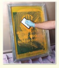
**Step 2.** Scrub screen with a non-abrasive pad or brush until all ink is completely liquified.
