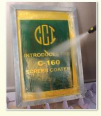
**Step 3.** High pressure rinse the screen starting at the bottom. Reverse screen and high pressure rinse. Continue washing off any blockout that remains.
