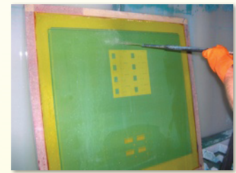
3. High pressure rinse - starting at bottom.
