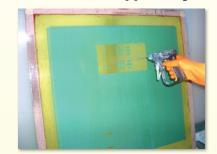
Step 1. After removal of ink, blockout, and tape, apply ER/80 to a wet screen(both sides).
