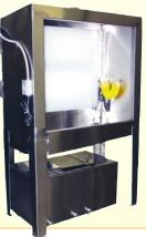
**RECIRCULATING WASH:** Card excessive ink from the screen. This product can be continuously recirculated until product becomes too heavily soiled with solids. Used product may be filtered and reused.
